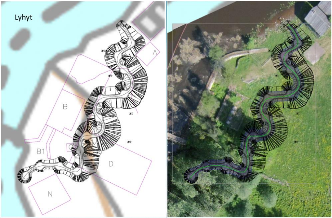
Fig 6. Fishway plan on the eastern side of the Koskenkoski Dam. (Jami Aho)
